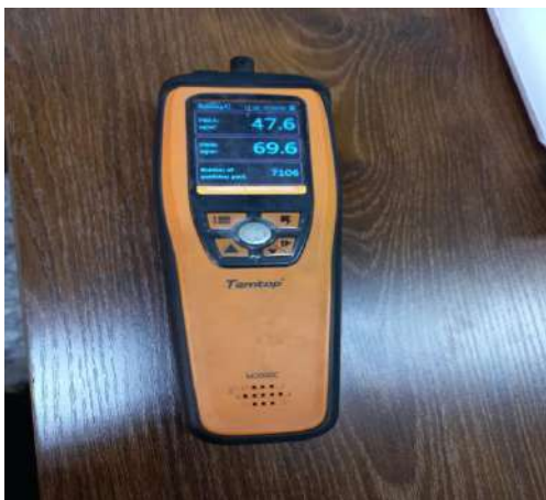
Figure 1- Portable particle mass counter device
