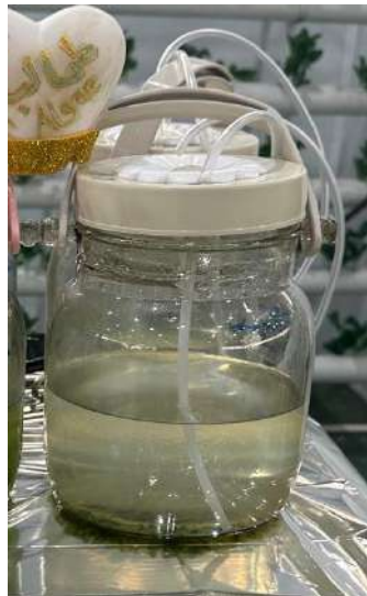
Figure 1- A simple photoreactor
